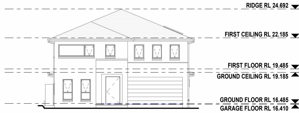
2 FRONT (EAST) ELEVATION 1 : 200
